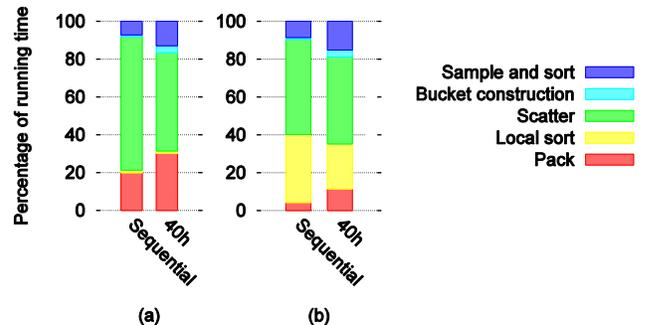
**Figure 3: Breakdown of the different phases in terms of percentage of the total running time for running sequentially and on 40 cores with hyper-threading (40h). The input has  $10^8$  records and the keys follow: (a) exponential distribution with parameter  $\lambda = 10^5$ , (b) uniform distribution with parameter  $N = 10^8$ . The data for this figure is taken from Table 2 and 3.**
