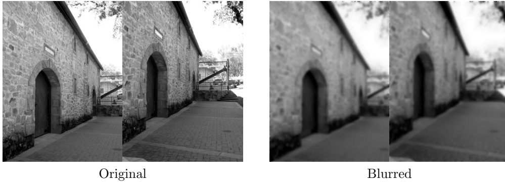
Figure 12.5 The photos on the left can be hard to align using automatic methods because they have lots of high-frequency detail that can obscure larger alignment patterns; by blurring the photos we can align larger features before refining the alignment using texture and other detail.
