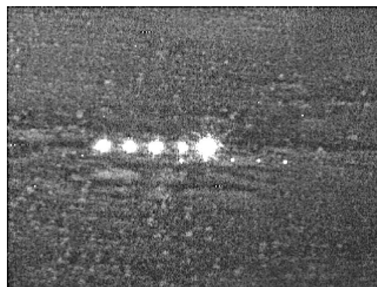
Fig. 1. Five laser beams incident on a dirt road, located 10 m in front of the vehicle. Image was captured with a SWIR camera.
