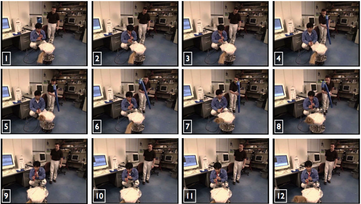
Figure 8-3: Fear Conditioning. This sequence of frames illustrates our first attempt toward affective learning. In this fear conditioning scenario, the robot is trained to predict the occurrence of the predator via a particular sound frequency.
