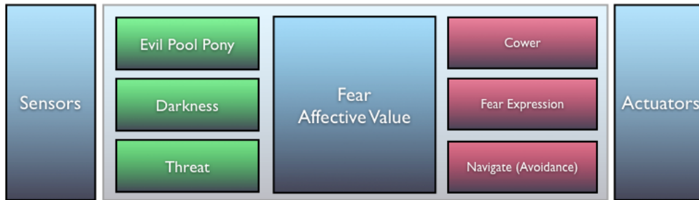
Figure 7-12: Illustration of an instance of the Fear Affect Program in the robot Yuppy. Three pathways were coordinated by Yuppy’s Fear Affective Evaluation mechanism. The first pathway mediates cowering responses that were evoked when the presence of Yuppy’s predator (the blue pool-pony) was detected. The second pathway involves the regulation of expressive behavior as it pertains to fear. Any threatening stimulus (i.e., blue pool-pony or darkness) would elicit a fearful expression to different extents. The final pathway regulates navigation for the robot according to the level of brightness perceived by the robot’s vision systems. If the robot is headed toward a dark region, navigation is controlled so that the robot veers away from that region.
