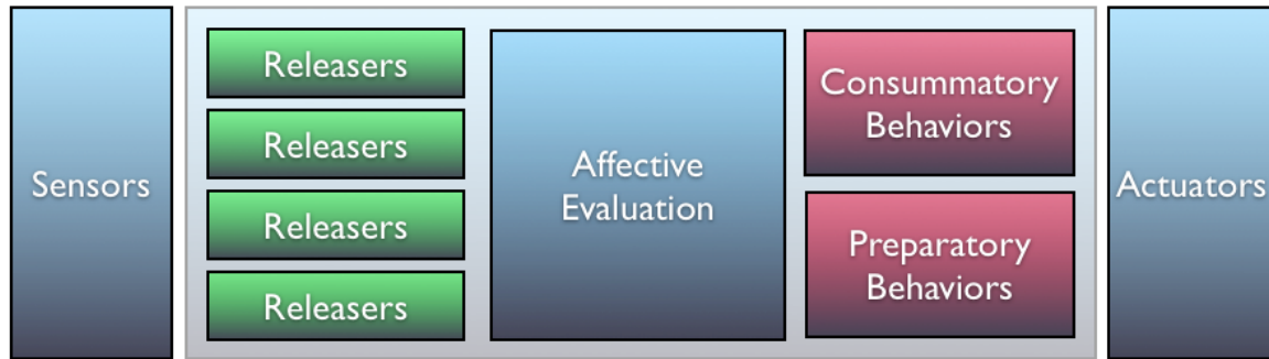
Figure 6-2: An abstraction for affect programs. This figure illustrates the main abstraction of the Cathexis framework: the Affect Program . An Affect Program couples sensors and actuators through affective processing. It consists of a set of filtering mechanisms, named Releasers , which provide information about the different stimuli in the robot’s environment, an Affective Evaluation Unit that assesses the affective significance of said stimuli and coordinates appropriate actions, named here as Preparatory and Consummatory Behaviors . Information through this affective processing mechanism flows from left to right.
