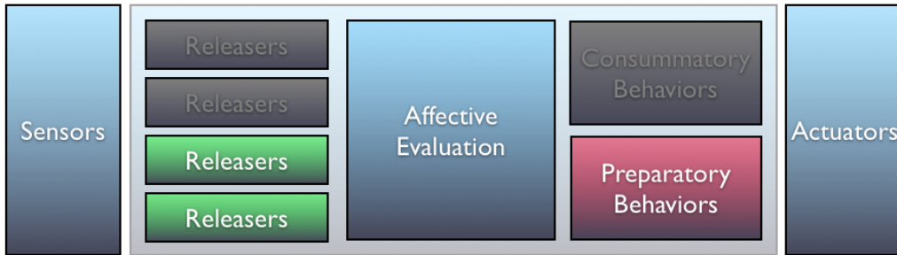
Figure 7-7: Pathway for Consummatory Behaviors. This figure illustrates the main organizational principle for action in the proposed framework as it relates to the notion of a separate sensorimotor pathway for consummatory behaviors that help bring the organism to be in proximal contact with goal objects, thus promoting survival.
