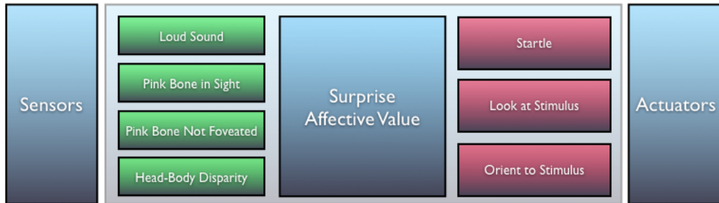
Figure 7-11: Illustration of an instance of the Surprise Affect Program in the robot Yuppy. Three main pathways were coordinated by Yuppy’s Surprise Affective Evaluation mechanism. The first pathway mediates startle responses due to the occurrence of high intensity sounds. The second pathway mediates Orienting Responses (OR) of the robot’s head to attend to and “foveate” the object of interest. The third pathway mediates full ORs that align the robot’s body and head so that it faces the object of interest, perhaps to initiate an approach response toward it.
