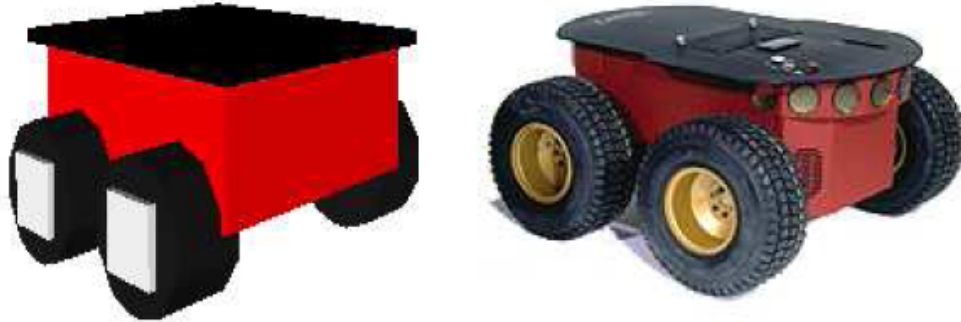
Figure 5-3: A Pioneer 2DX Robot in the Gazebo Simulator. Gazebo is a high fidelity robotics simulator for 3D environments that is capable of providing realistic sensor feedback as well as an accurate dynamic environment, such as those that physical robots would face in the real world. This figure illustrates how a physical robotic base such as the Pioneer 2DX system can be simulated in the this engine. Adapted from (Koenig & Howard, 2004)
