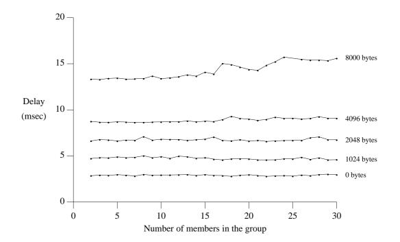
Fig. 3.21. Delay for 1 sender using the BB method.
