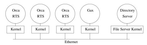
**Fig. 5.2.** An Amoeba system with an Orca application running on 3 processors. The Orca processes together form one process group. In the current configuration, the file server is for performance reasons linked with the kernel.
