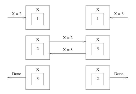
**Fig. 1.3.** Server 1 and 2 receive at approximately the same time an update message for the shared variable X. The copies of X become inconsistent because the messages from Server 1 and Server 2 are not ordered.
