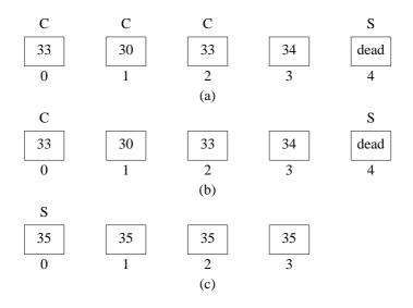
**Fig. 3.18.** A possible recovery for a group of size 5 after a crash of member 4. S is a sequencer. C is a coordinator. The number in the box is the sequence number of the last message received. The number below the box is the member id. (a) Shows a possible start of phase 1. (b) Shows the start of phase 2. In (c) the recovery has been completed.
