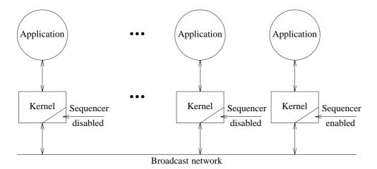
**Fig. 3.6.** System structure. Each node runs a kernel and a user application. Each kernel is capable of being sequencer, but, at any instant, only one of them functions as sequencer. If the sequencer crashes, the remaining nodes can elect a new one.
