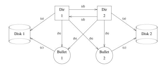
**Fig. 5.6.** The configuration. The boxes represent the directory servers, while the circles represent the Bullet file servers. The arrows imply the client/server relationship. (a) Administrative Data; (b) Directories; (c) Files; (d) Intentions and other internal messages.
