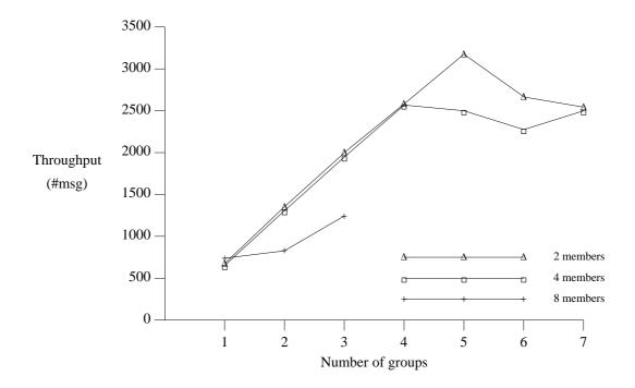
**Fig. 3.24.** Throughput for groups of 2, 4, and 8 members running in parallel and using the PB method. We did not have enough machines available to measure the throughput with more groups with 8 members.
