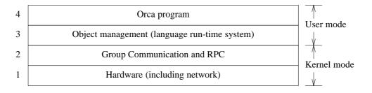
Fig. 4.6. Layers in the shared data-object model.
