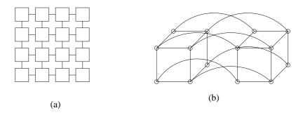
Fig. 4.5. Multicomputers. (a) Grid. (b) Hypercube.
