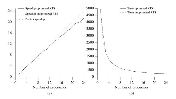
**Fig. 4.14.** Performance for the All-Pairs Shortest Paths Problem using a graph with 500 nodes. (a) Speedups for each implementation of the RTS. (b) Absolute running times in seconds for each implementation of the RTS.
