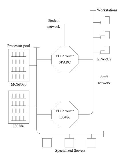
**Fig. 2.8.** The FLIP internetwork at the Vrije Universiteit. It contains three different machine architectures with different endianness and two types of networks: Ethernet and VME-buses. On average ten people are using the Amoeba system every day to develop system software, and distributed and parallel applications.
