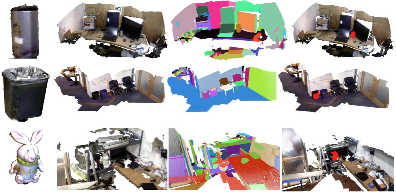
Fig. 7. Left column: Objects discovered from changes in previous maps (not shown). Center left column: New maps with the discovered objects in them. Center right column: Random colored segmented versions of the map using the optimized segmentation method and parameters for each specific object. Right column: Original map with object segment detected and highlighted in red. From top to bottom, the objects are a jar, a trash bin, and a stuffed bunny respectively. The detections were automatically trained using from one, two, and four objects for the jar, trash bin, and bunny respectively. Note the trash bin in the second row map is detected, and not the similarly proportioned by different colored recycle bin next to it.
