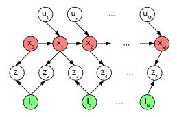
Fig. 1. Bayesian belief network representation of the SLAM problem,  $\mathbf{x}_i$  is the state of the robot at time i,  $\mathbf{l}_j$  the location of landmark j,  $\mathbf{u}_i$  the control input at time i and  $\mathbf{z}_k$  the  $k^{th}$  landmark measurement.
