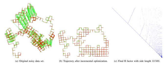
Fig. 9. iSAM results for the simulated Manhattan world from [21] with 3500 poses and 5598 constraints. iSAM takes about 40ms per step. The resulting R factor has 187423 entries, which corresponds to 0.34% or an average of 17.8 entries per column.
