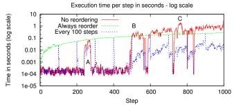
(d) Execution time per step for different updating strategies are shown in both linear (top) and log scale (bottom).
