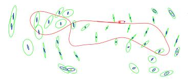
Fig. 7. Comparison of marginal covariance estimates *projected into the current robot frame* (robot indicated by red rectangle), for a short trajectory (red curve) and some landmarks (green crosses). Conservative covariances (green, large ellipses) are shown as well as the exact covariances (blue, smaller ellipses) obtained by our fast algorithm. Note that the exact covariances based on full inversion are also shown (orange, mostly hidden by blue).
