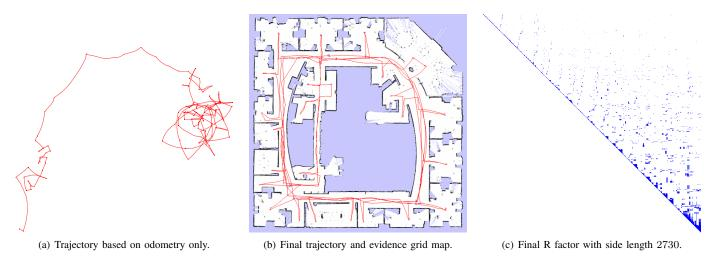
Fig. 10. Results from iSAM applied to the Intel dataset. iSAM calculates the full solution for 910 poses and 4453 constraints with an average of 85ms per step, while reordering the variables every 20 steps. The problem has  $910 \times 3 = 2730$  variables and  $4453 \times 3 = 13359$  measurement equations. The R factor contains 90363 entries, which corresponds to 2.42% or 33.1 entries per column.
