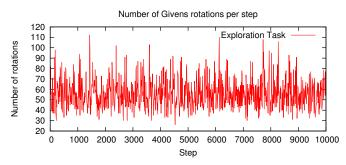
Fig. 4. Number of Givens rotations needed per step for a simulated linear exploration task. In each step, the square root factor is updated by adding the new measurement rows by Givens rotations. The number of rotations is independent of the length of the trajectory.
