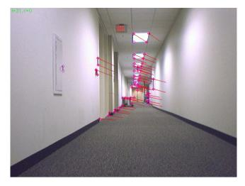
Figure 7: Camera image with measurements and reprojected structure.
