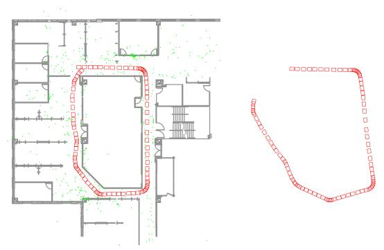
(a) Final trajectory and map (left) and trajectory based on odometry only (right).
