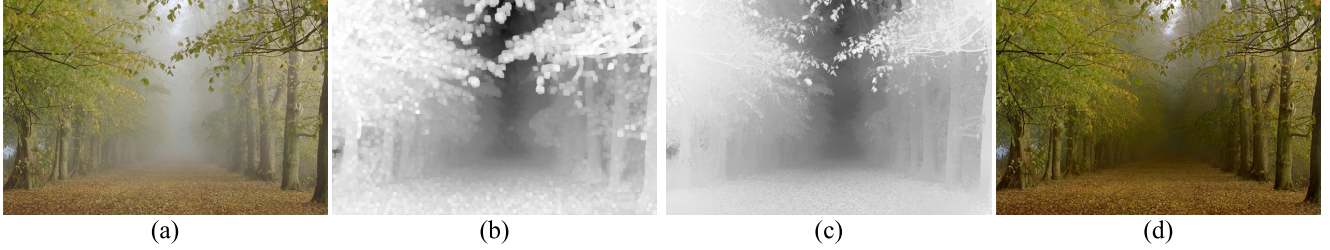
Figure 5. Haze removal result. (a) input haze image. (b) estimated transmission map. (c) refined transmission map after soft matting. (d) final haze-free image.
