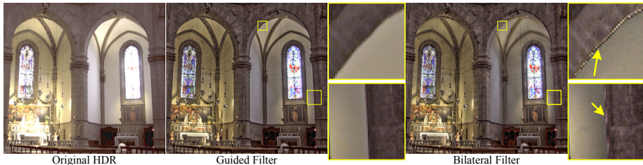
Fig. 7. HDR compression. The parameters are r = 15 , \epsilon = 0.12^2 for the guided filter, and \sigma_s = 15 , \sigma_r = 0.12 for the bilateral filter.
