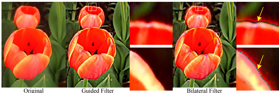
Fig. 6. Detail enhancement. The parameters are r = 16 , \epsilon = 0.1^2 for the guided filter, and \sigma_s = 16 , \sigma_r = 0.1 for the bilateral filter. The detail layer is boosted \times 5 .
