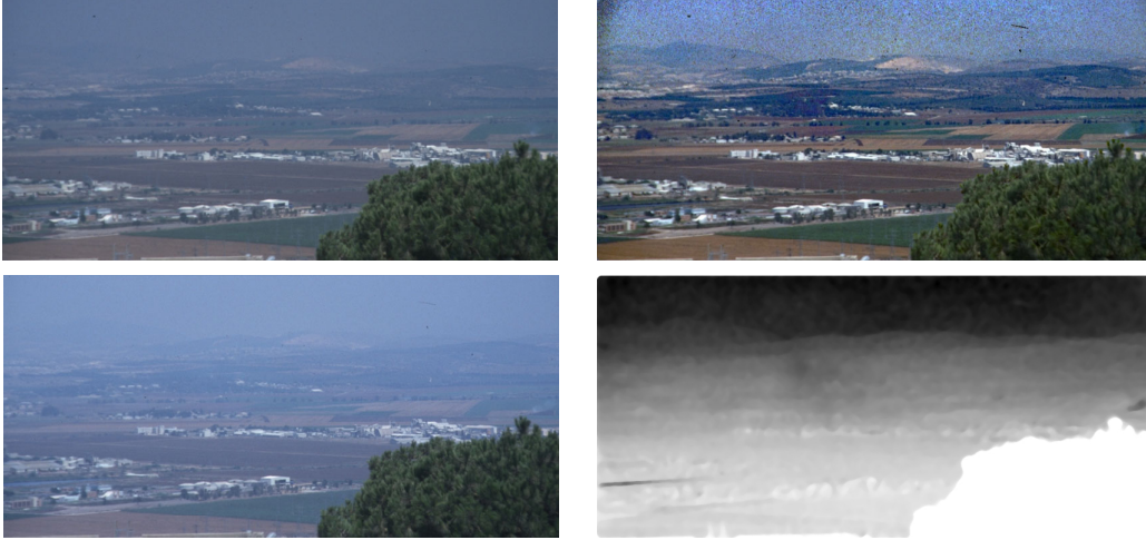
Figure 2.7: Polarization-based methods. On the left are two images taken in two polarizer states. On the right are the estimated scene radiance and depth. Images from [65].
