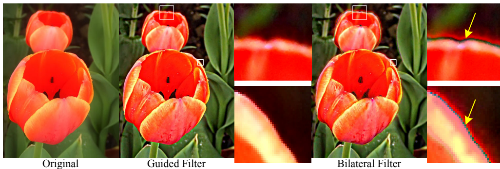
Figure 4.16: Detail enhancement. The parameters are r = 16 , \epsilon = 0.1^2 for the guided filter, and \sigma_s = 16 , \sigma_r = 0.1 for the bilateral filter. The detail layer is boosted \times 5 .
