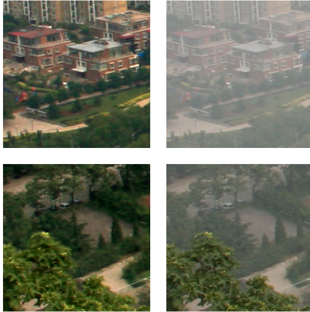
Figure 2.3: Images degraded by haze. On the left are the scene radiance \mathbf{J} . On the right are the observed hazy images \mathbf{I} .
