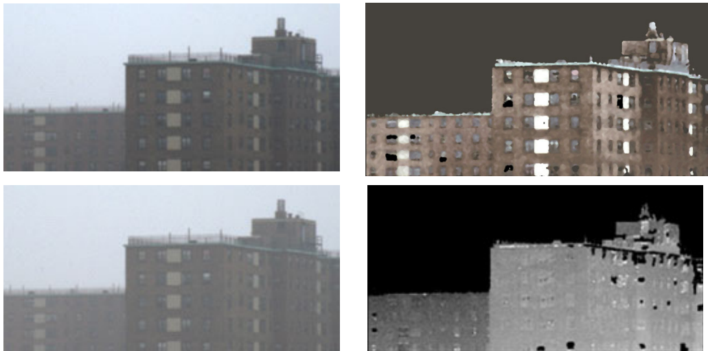
Figure 2.6: Haze removal based on varying atmospheric conditions. On the left are two images taken in two hazy conditions. On the right are the estimated scene radiance and depth (the sky is ignored). Images from [48].
