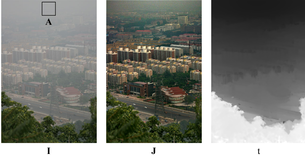
Figure 2.1: Variables in the haze imaging equation. The transmission map t is shown as white when t=1 , and black when t=0 .
