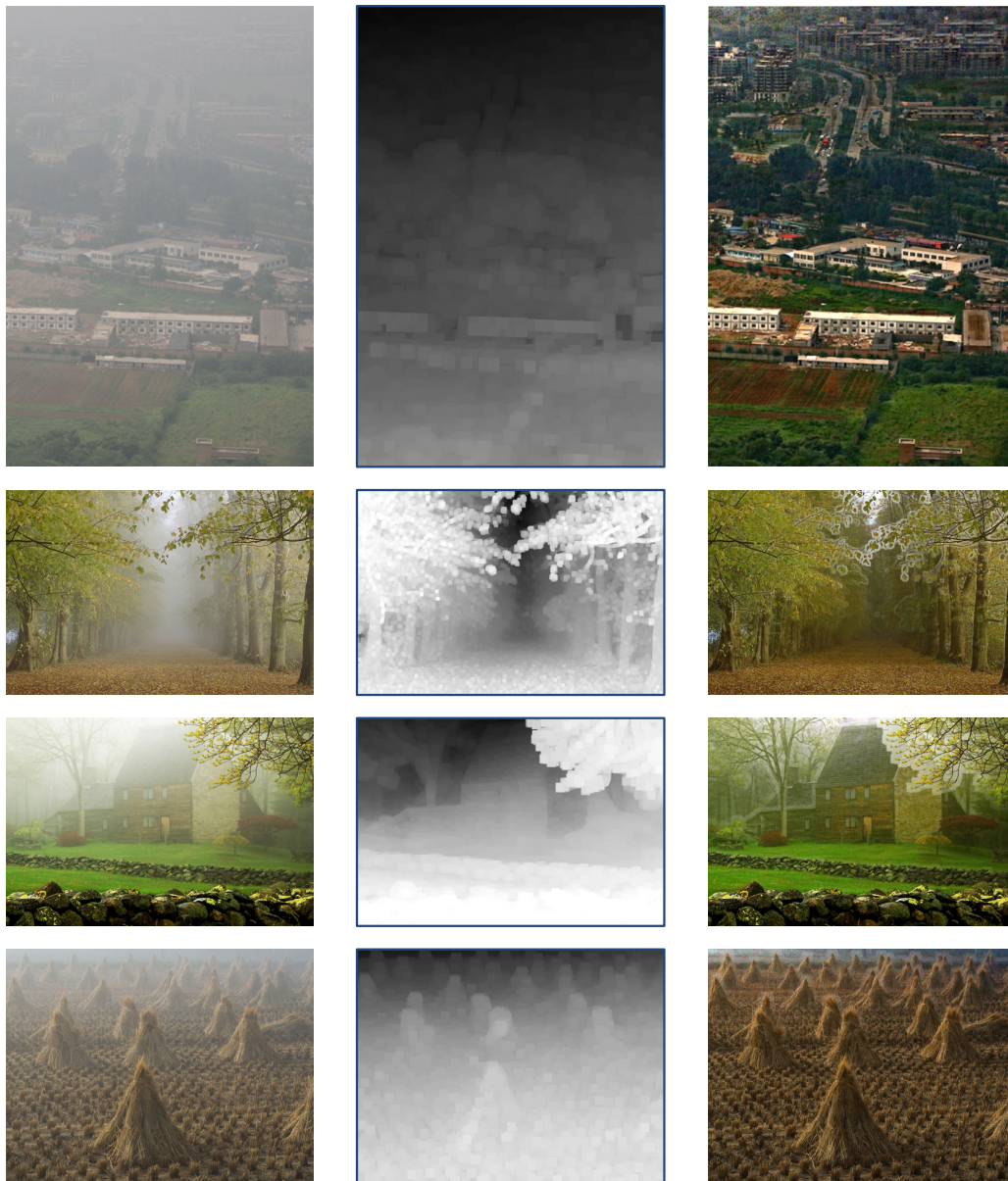
Figure 3.6: Haze removal using Equation (3.14). Left: input hazy images. Middle: transmission maps estimated by (3.14). Right: recovered scene radiance by these transmission maps.
