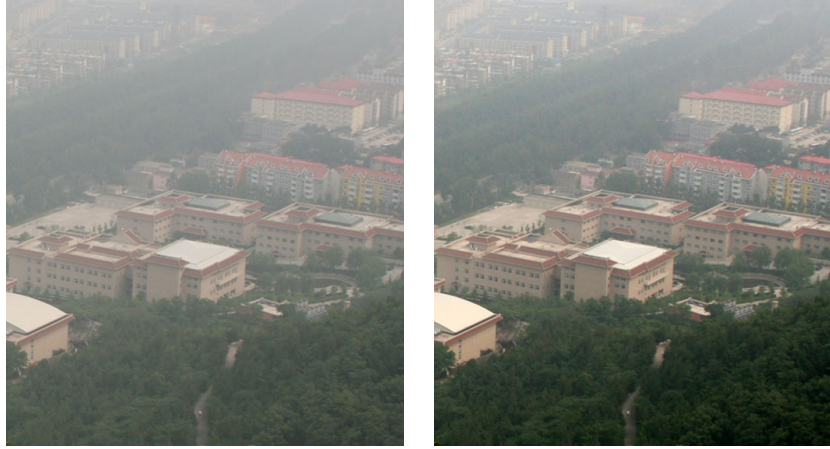
Figure 2.9: Haze removal by dark object subtraction [9]. Left: input hazy image. Right: haze removal result.
