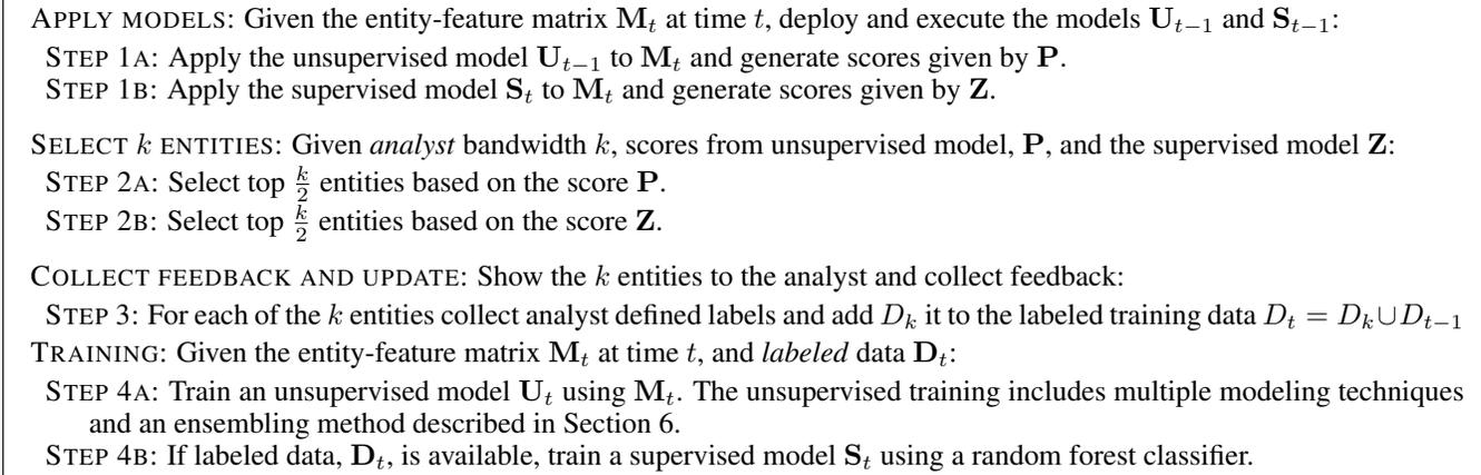
Figure 10: ACTIVE MODEL SYNTHESIS algorithm
