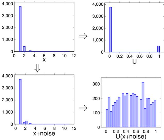
Figure 7: A discrete valued variable will not have a *uniform* density for its *cdf* values (top right). However, if tiny amount of additive white Gaussian noise is added to the variable (essentially making it continuous), the density of its *cdf* values look closer to *uniform* (bottom right). We use this trick to be able to model discrete variables using copulas.
