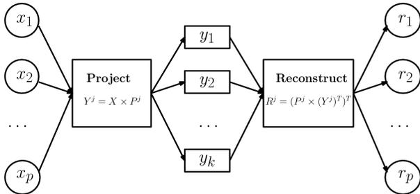
Figure 5: Matrix Decomposition outlier detection method: the original variables are projected into the top  $j$  principal components space. The dataset is reconstructed with the inverse projection, and the reconstruction error is used as the outlier score.
