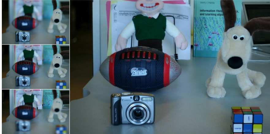
Fig. 10 Three images (left) were taken, focused in objects in foreground (top), middle ground (middle), and background (bottom), and combined into a single image that is sharp everywhere (right). Image by Daniel Vaquero.
