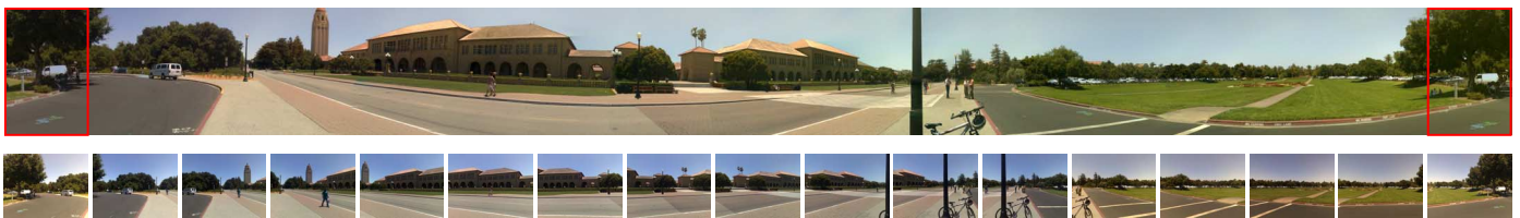
Fig. 4. Color differences between the first and last areas of a 360-degree panoramic image.
