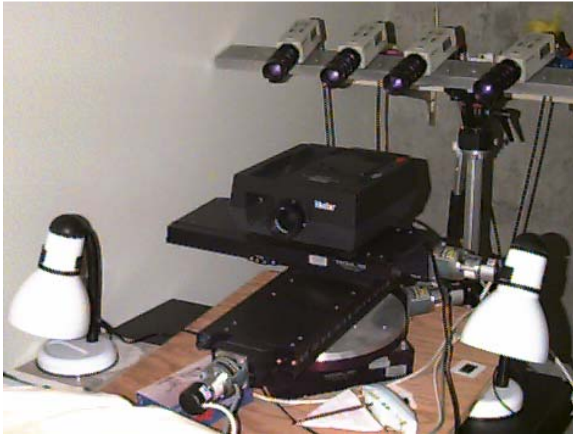
Figure 2-1 The scanner hardware. Four video cameras are attached to an aluminum bar, which rests on a tripod. A slide projector is placed on a turntable under the cameras. Table lamps provide adjustable lighting for capturing color images.
