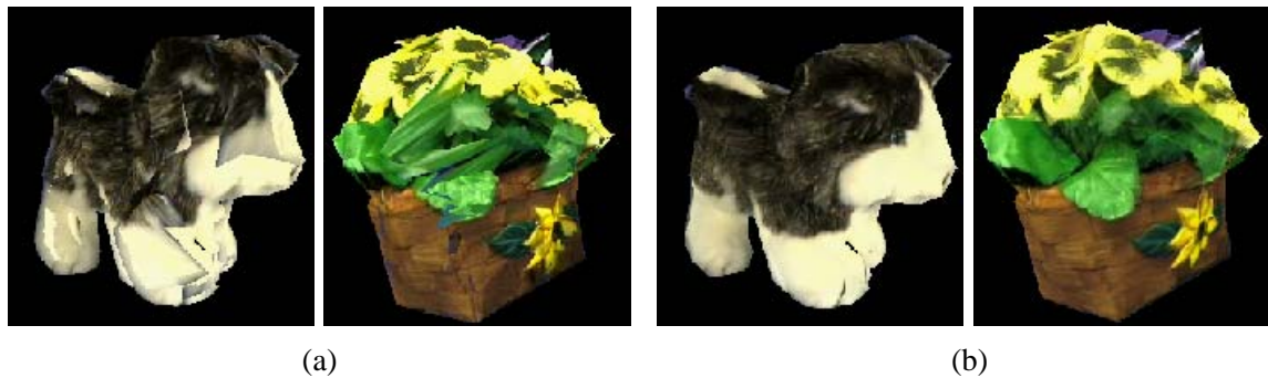
Figure 5-16 (a) The result of combining three views by rendering each of the view-based meshes from the viewpoint of the virtual camera. (b) Using the three weights and soft z-buffering produces a much better result.
