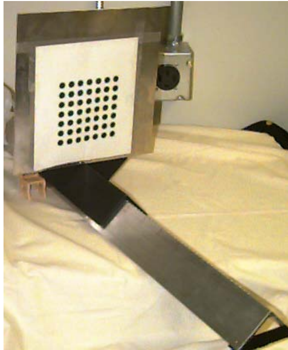
Figure 2-2 The calibration object is metal plate mounted on a rail. The plate is perpendicular to the rail, and it can be moved in 10 mm steps along the rail. A calibration pattern consisting of a 7 \times 7 dot field is pasted on the plate.
