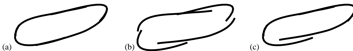
Figure 3-16 (a) A scanned object. (b) Initial registration of the views. (c) Errors in pairwise registrations accumulate.
