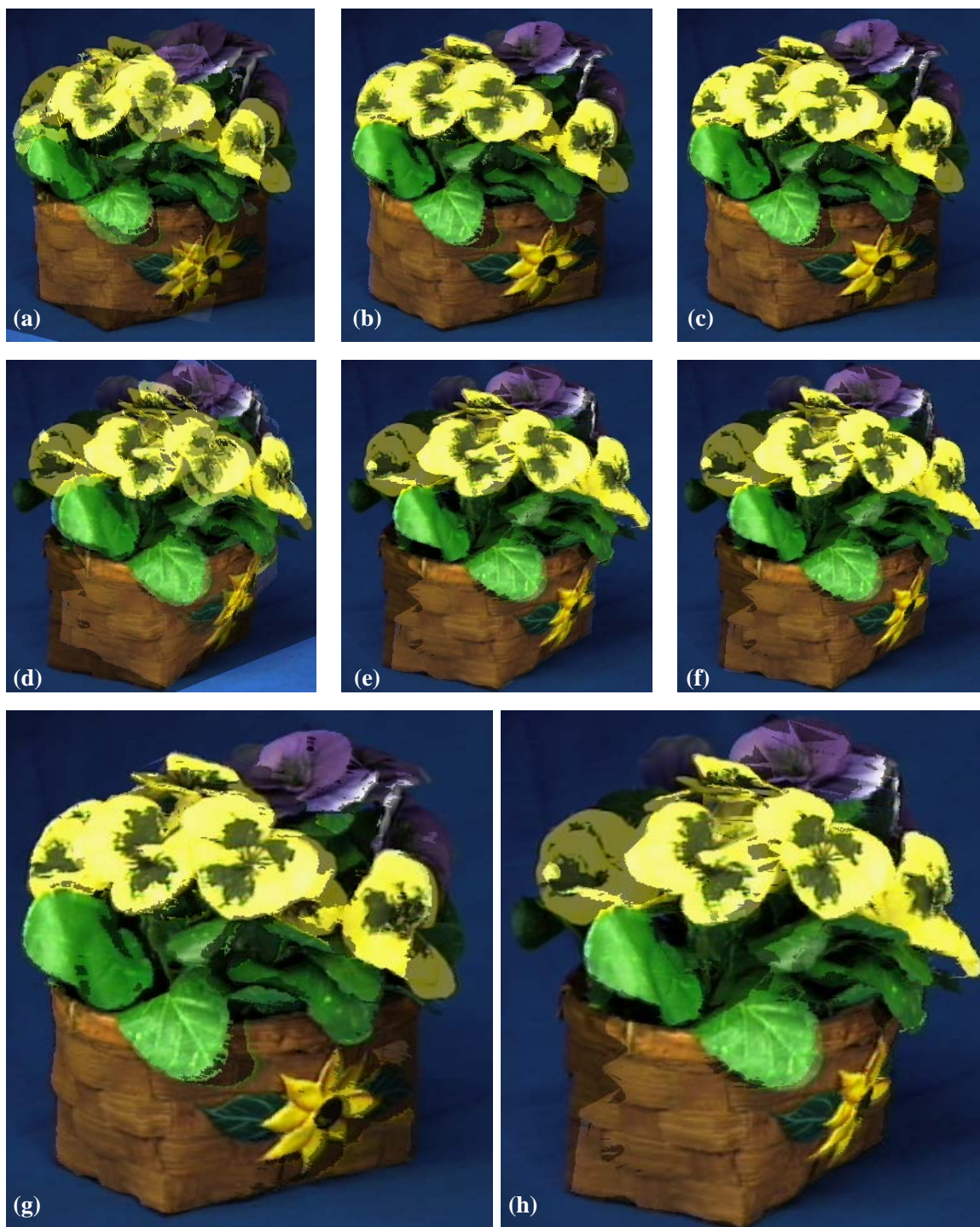
Figure 3-13 Registration results of the new method. Images (a), (b), (c), (g) form a sequence as seen from one camera, (d), (e), (f), (h) as seen from the other camera. (a) & (d) The result of 2D image registration from Fig. 3-12. (b) & (e) The result after a 3D registration is found using the point pairs found through 2D registration. (c) & (f) The result of 2D registration on images (b) and (e). (g) & (h) The final result after 3 iterations.
