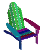
Figure 3-1 The range maps are registered by aligning the range data in the different views, each expressed in the sensor coordinate system. Registration of the data is equivalent to finding the rigid transformations of the sensor between the scans.
