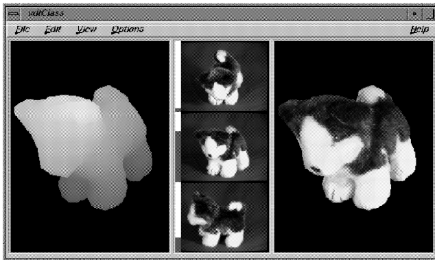
Figure 9. Our interactive viewer. Left: the colors code the visible surface points. Middle: the three views that have been chosen as inputs, along with bars that show the directional weight. Right: the final image.
