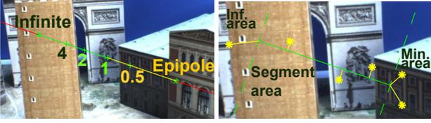
Figure 3. **Left:** the epipolar segment goes from the projection of the point with minimum depth to that of the point with infinite depth. **Right:** the distance measure has three areas: distance to the line, distance to the minimum depth projection, and distance to the infinite depth projection.
