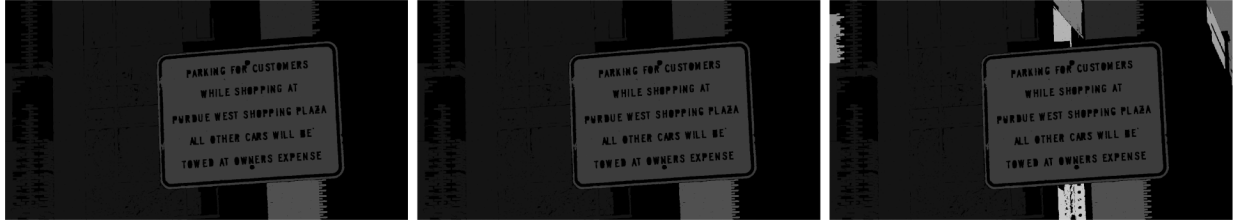
Fig. 7. Segmented potential sign backgrounds found at various block sizes, K = 32, 16, 8 (left to right). Non-black regions are considered homogeneous. Each shade of gray corresponds to one region.
