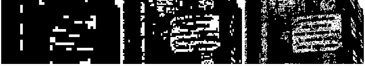
Fig. 5. Homogeneous block selection for the image in Fig. 2 using various block sizes, k = 32, 16, 8 (left to right). Homogeneous regions are shown as white areas. As K decreases, more homogeneous blocks are detected.
