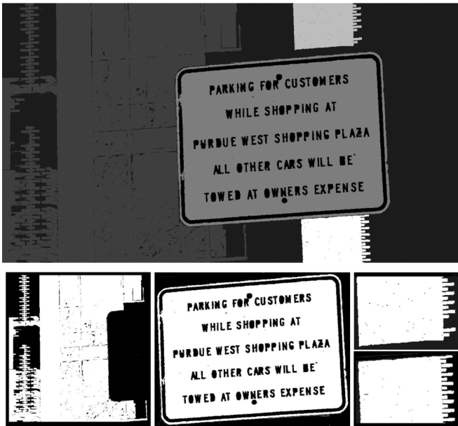
Fig. 8. Isolating regions of an image. (Top) Regions of an image. (Bottom) Isolated regions of the image enclosed by exaggerated bounding regions. Potential sign background regions are white and background regions are black.
