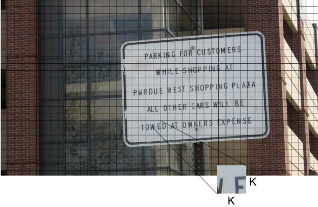
Fig. 2. Input image divided into a grid of K \times K -pixel blocks. Each pixel block is tested for homogeneity to determine if it is part of the background of a sign.
