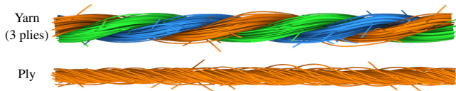
Figure 2: Yarn structure: Yarn typically consists of multiple plies, each of which is made up of tens to hundreds of micron-diameter fibers, depending on the yarn type.
