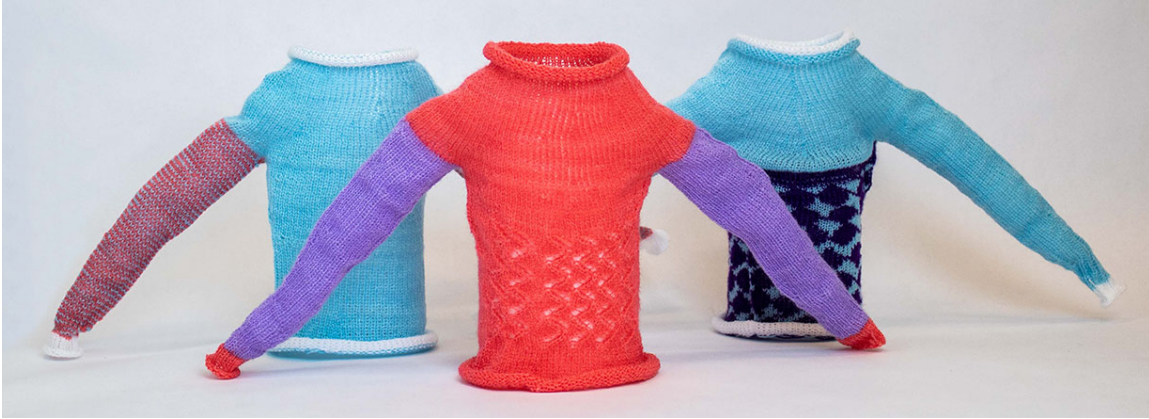
Fig. 5.15: Multiple variations – including lace (center) and colorwork (intarsia stripes left, Fair Isle right) – on the same base pattern can be easily introduced.
