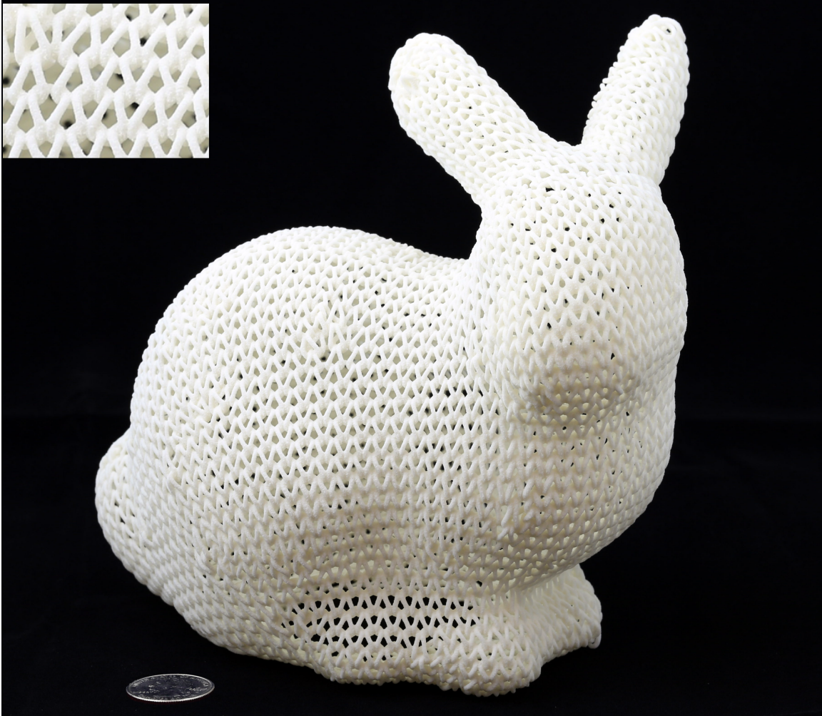
Fig. 3.26: A knitted “bunny” model generated with our pipeline and printed using selective laser sintering.
