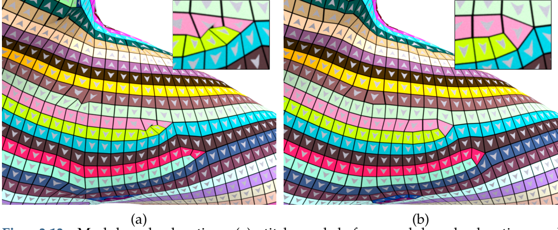
Fig. 3.13: Mesh-based relaxation: (a) stitch mesh before mesh-based relaxation, and (b) stitch mesh after mesh-based relaxation.
