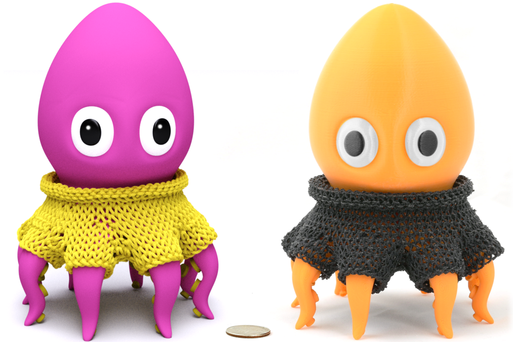
Fig. 3.24: An octopus wearing a knitted sweater: (left) simulated model and (right) fabricated via 3D printing.
