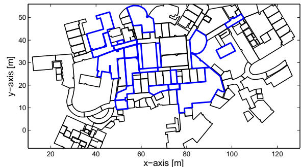
Fig. 1. During the growth phase of an organic positioning system, not all rooms have been surveyed by users, confounding localization in unsurveyed rooms. Spaces outlined in blue are represented in our fingerprint database.
