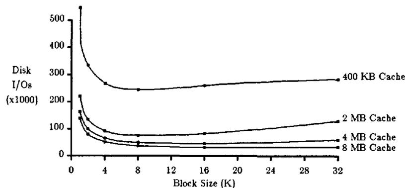
**Figure 6.** Disk traffic as a function of block size and cache size, for the A5 trace using the delayed-write policy. Large block sizes work well for small caches, but they work even better for large caches. For very large block sizes, the curves turn up because the cache has too few blocks to function effectively as a cache.
