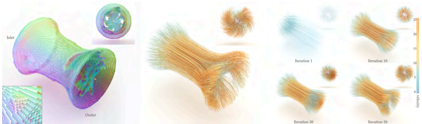
Fig. 1. We present a topology optimization pipeline for designing Stokes-flow fluidic systems with flexible and accurate boundary conditions. Our method automatically creates the structure of this fluidic twister on an 100 \times 100 \times 100 grid after optimizing nearly four million decision variables. The goal of this device is to generate a swirl flow at its outlet given a constant inflow. Left: our final design is made of spatially-varying anisotropic materials, which we visualize as a small disk in each voxel colored based on its anisotropic direction (bottom-left inset). Our method automatically synthesizes a propeller-like structure (top-right inset) to facilitate the vortex generation near the outlet. Middle: the flow simulated from the final design, visualized as streamlines. A vortex emerges near the outlet (top-right inset). Right: visualization of flows from the fluidic device after 1, 10, 20, and 50 iterations of topology optimization.
