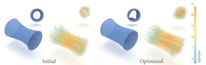
Fig. 10. Solving the Fluidic Twister example using the open-source implementation from Du et al. [2020]. Left: The parametric shape and fluid flow visualization before optimization, with the top-right insets showing the designs viewed from their outlets. Right: The corresponding visualizations after optimization.
