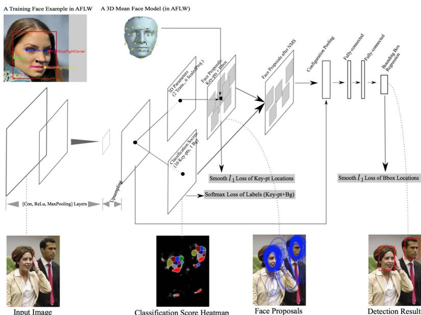
Figure 1: Illustration of the proposed method (Top), and a sample intermediate and the final detection results (Bottom).
