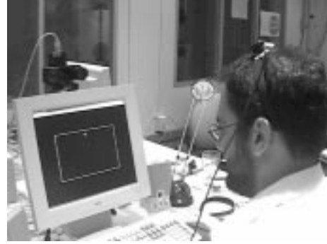
Figure 2. A user during the desktop experiment. The SRI stereo camera is placed just over the screen and the user is wearing the Intertrax 2 device on his head.
