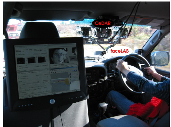
Figure 1: The vision platforms in the vehicle. The CeDAR active vision head and FaceLAB passive stereo cameras are labelled.
