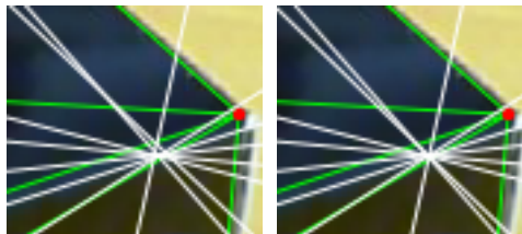
Figure 3.11: Illustration of the effect of enforcing the singularity constraint (magnified); non-singular fundamental matrix F on the left, singular F on the right.
