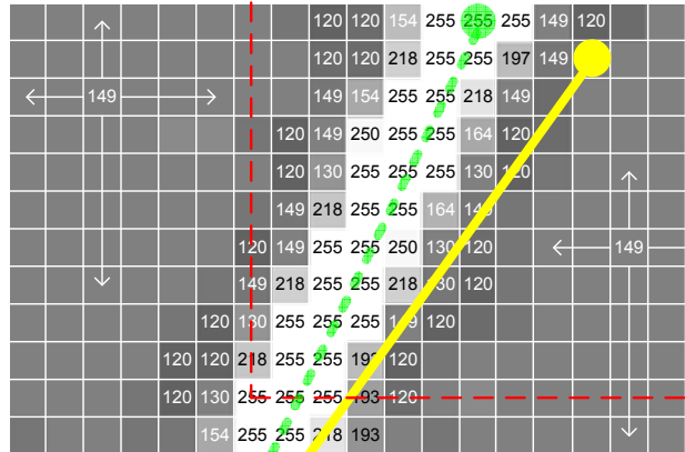
Figure 3.8: Schematic view of the snapping calculations. The dashed red line is the boundary of the snapping window, the green line is the line corresponding to the optimal snapping score, the yellow line is where the user is pointing.
