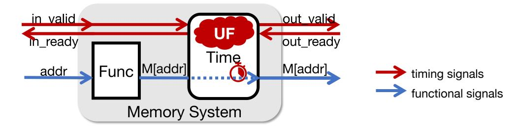
Pensieve uses **simple** models with **UF** to cover **space** of microarchitectures with **complex** timing behaviors
