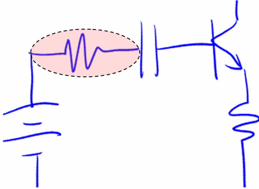
Figure 3-2: An example showing a multi-object stroke. The selected circuit fragment contains two wires and a resistor drawn using a single stroke.
