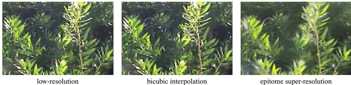
Figure 4. Video super resolution. (Left) A single frame from a low resolution 135 \times 90 \times 32 sequence. (Middle) The 360 \times 240 bicubic interpolation of the frame. (Right) The 360 \times 240 video epitome super-resolution result. A 325 \times 225 \times 8 video epitome was learnt from a 360 \times 240 \times 17 high resolution sequence captured when the camera physically zoomed into a similar scene at a different point in time. Super-resolution was performed by reconstructing the low resolution sequence with the epitome containing the features from the high resolution sequence. Video cubes of size 75 \times 75 \times 4 , 50 \times 50 \times 3 , and 25 \times 25 \times 2 were used during learning and reconstruction. The video of this super-resolution result is available at http://www.psi.toronto.edu/~vincent/videoepitome.html .
