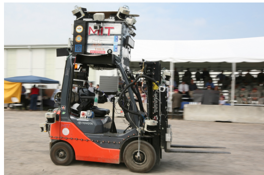
Fig. 5. The robotic forklift used for experimental validation.
