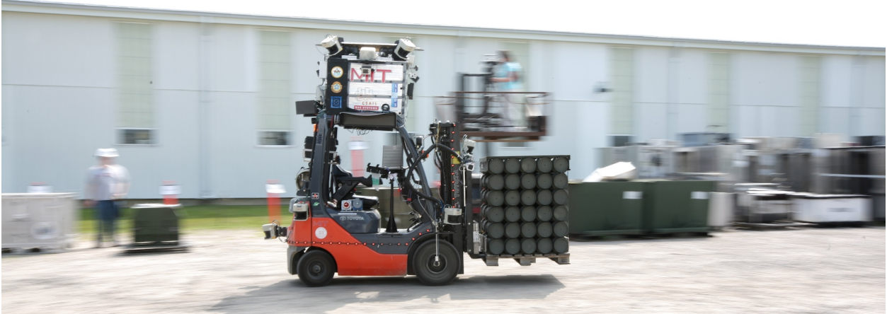
Figure 9: The robot transporting cargo at an active military outdoor storage facility.
