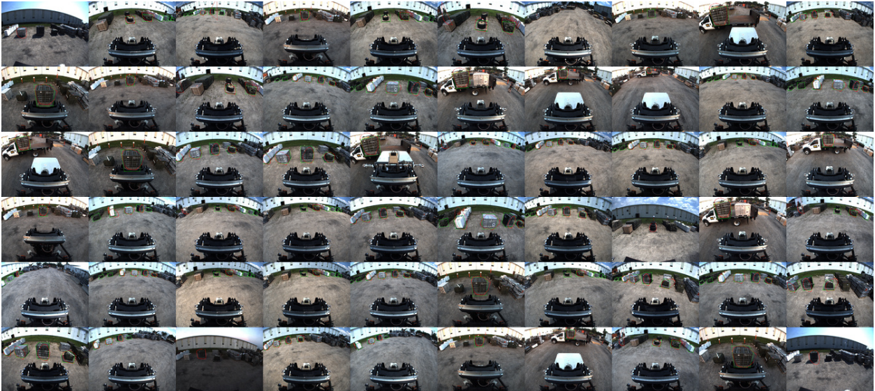
Figure 10: Some of the images acquired from the forward- and right-facing cameras during the five scenarios of the experiment. The right-facing images (those without the forklift structure in the lower portion of the frame) reveal the user gestures that indicate the sole training example for each object. The forward-facing images show model views learned automatically by the algorithm with their reconstituted gestures (red, ellipse-like outlines).
