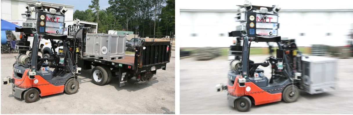
Figure 1: The robotic forklift is capable of autonomously manipulating and transporting cargo based upon image-space segmentation and voice commands.
