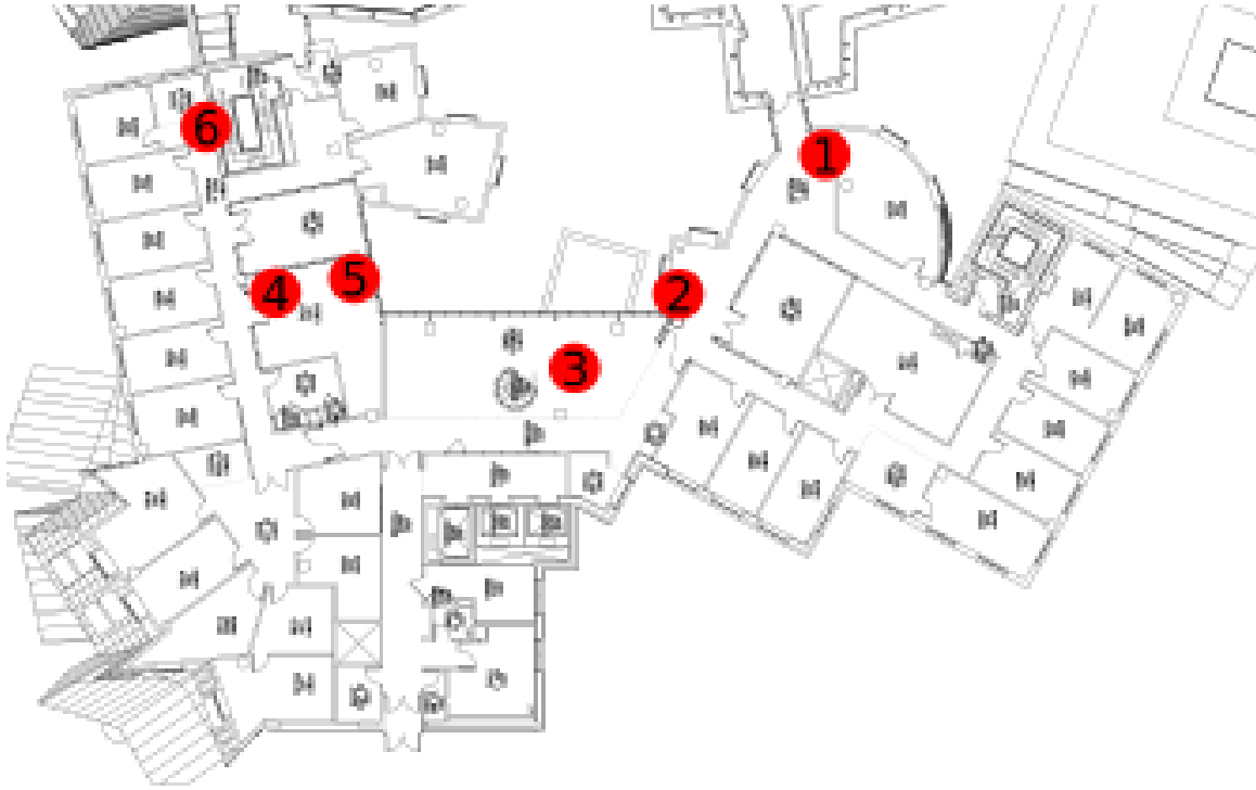
Figure 5-4: Raspberry Pi Placement in 6th Floor Building 32 at MIT
