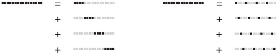
Figure 5: Two ways to map lattice data into memory. (a) The direct partition used in the previous Figure. Bit-field bits belonging to consecutive lattice sites are stored together in words of memory. (b) Bits spread evenly across the space are stored together in memory words. Each 4-bit memory word holds a uniform *skip-sample* of an entire bit-field.
