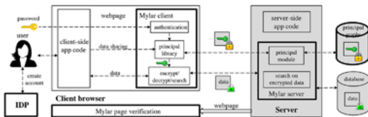
Figure 1: System overview. Shaded components have access only to encrypted data. Thick borders indicate components introduced by Mylar.
