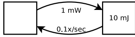
Figure 2: A common idiom in Cinder. The reserve on the left sources 1 mW of energy to the reserve on the right. Unused energy is taxed at a rate of 10%/sec and returned to the reserve on the left. The right reserve, while unused, converges on 10 mJ naturally as a product of the in and out taps.
