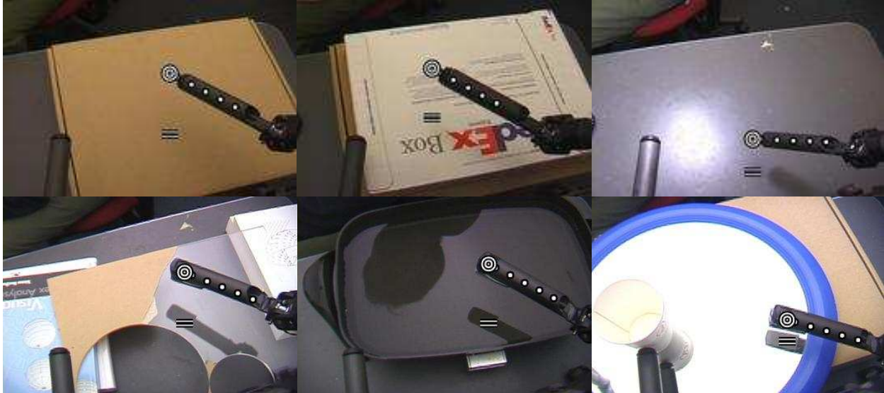
Figure 11: In our work on reaching, we detect the endpoint of the arm (circle and white dots) and the shadow it throws (bar) using motion cues (Fitzpatrick and Torres-Jara, 2004) Changes in the distance to the shadow (or reflection) of the robot arm are interpreted as changes in the distance to the surface.
