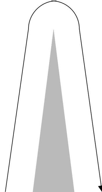
Robot cannot turn an arc with a radius less than the robot itself.
