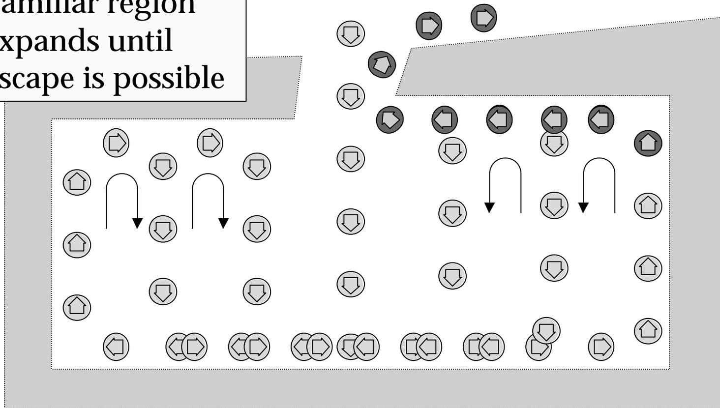
Robot uses “familiarity” sensor to escape from trap.
