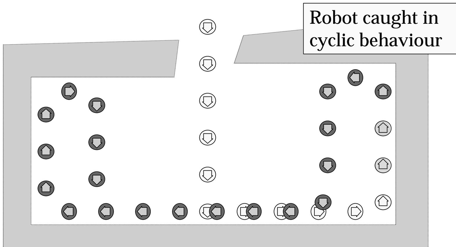
Robot shown trapped by an awkwardly shaped obstacle.
