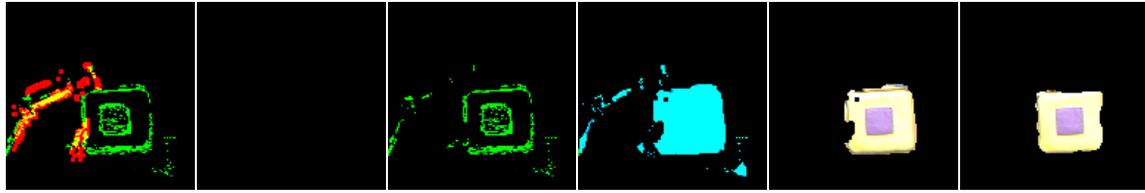
*Motion in frame immediately after impact*   *Aligned motion from before impact*   *Masking out prior motion*   *Result of segmentation*   *Largest connected region found*   *Refinement of segmentation*
