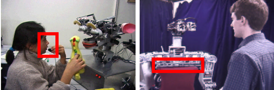
Figure 9-1: For Kismet, a clip-on/hand-held microphone was used (left). Anyone interacting with the robot needed to be informed of this. Experience showed that people would frequently forget to use the microphone if it was not clipped on – it was not an intuitive interface for face-to-face communication. On Cog, a commercial microphone array was installed (right), with a clip-on microphone available for when there was excessive background noise – Cog is located right beside a busy machine shop. This meant that the robot could always respond to voice in its vicinity, and if its responses were poor, the human could either move closer, speak louder (natural responses) or pick up the back-up microphone. The transition between microphones is handled automatically.
