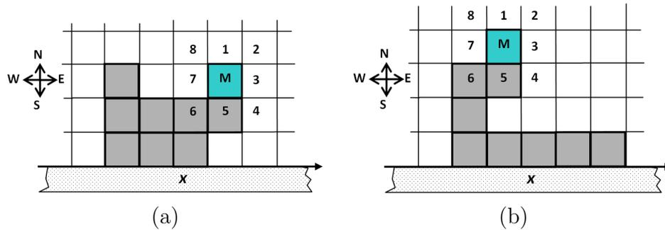
Figure 4-5: Two global configurations that are aliased assuming only local, partial observations, even in the presence of directional information: (a) module  $M$  is really at the front of the robot and should not move, (b) module  $M$  should be able to move despite having no “front” neighbors.
