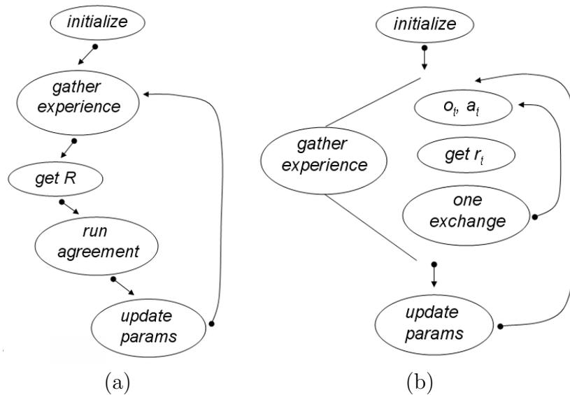
Figure 5-2: Two implementations of agreement exchanges within the GAPS learning algorithm: (a) at the end of each episode, and (b) at each time step.
