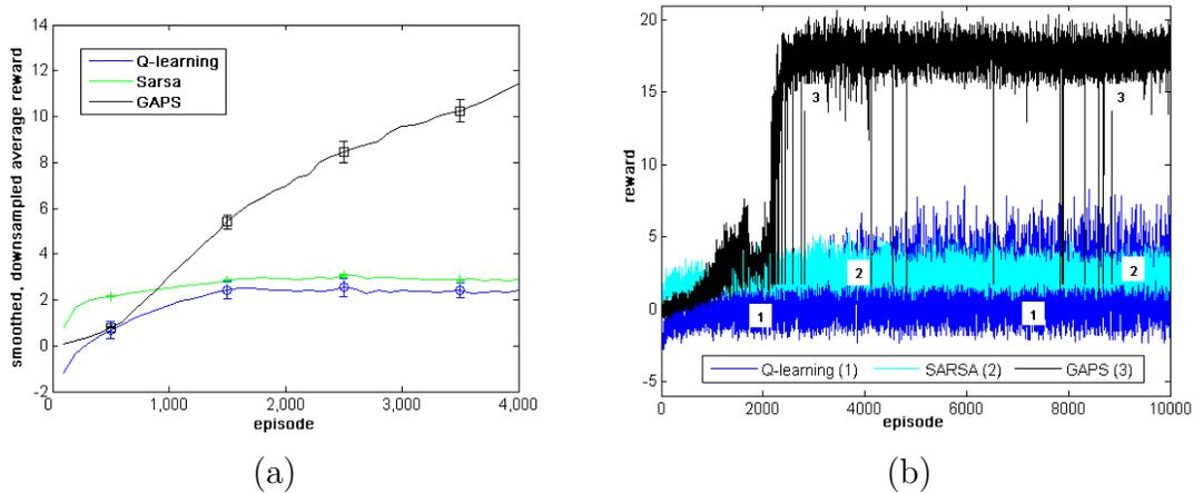
Figure 3-3: Performance of policies learned by 15 modules in the 2D locomotion task running Q-learning, Sarsa and GAPS: (a) smoothed (100-point moving window), downsampled average rewards per learning episode over 10 trials (Q-learning and Sarsa each), 50 trials (GAPS), with standard error (b) typical single trial learning curves.
