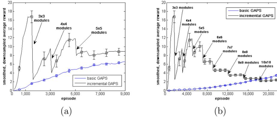
Figure 4-8: Incremental learning by square side length: smoothed, downsampled average rewards for (a) 25 and (b) 100 modules learning eastward locomotion with basic vs. incremental GAPS. Rewards obtained in 50 timesteps by basic GAPS are greater than those of incremental GAPS for 100 modules; this highlights the effect of shorter episode lengths on learning, as policies learned by incremental GAPS are much more likely to be locomotion gaits (see text and table 4.3.5).
