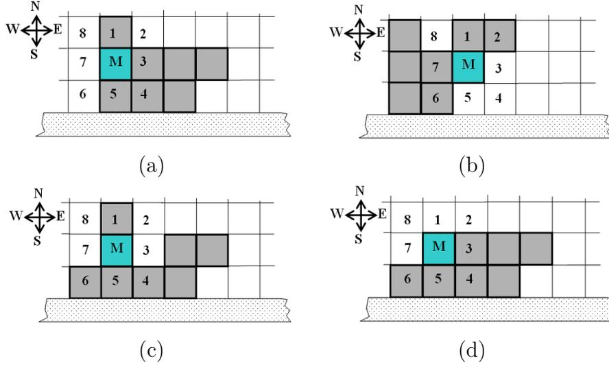
Figure 4-1: Determining if actions are legal for the purpose of constraining exploration: (a)  $A = \{NOP\}$ , (b)  $A = \{NOP\}$ , (c)  $A = \{NOP\}$  (d)  $A = \{2(NE), 7(W)\}$ .
