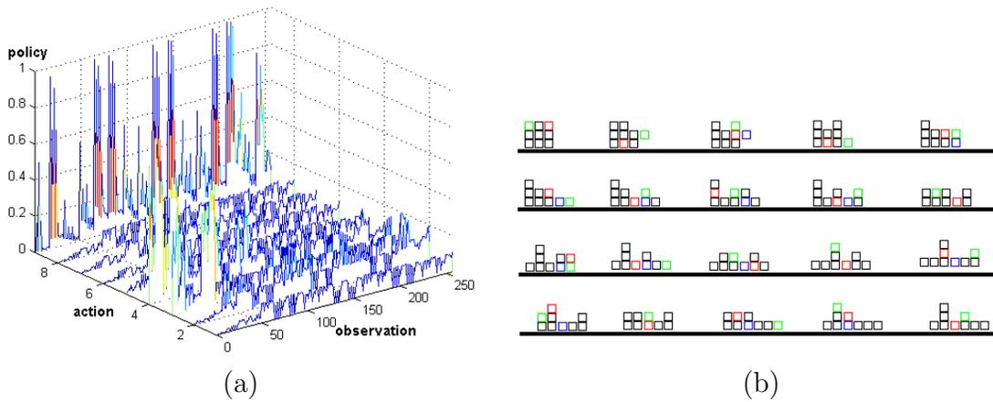
Figure 3-2: (a) A locomotion gait policy (conditional probability distribution over actions given an observation). (b) First few configurations of 9 modules executing the policy during a test run: in blue, module with lowest ID number, in red, module which is about to execute an action, in green, module which has just finished its action.
