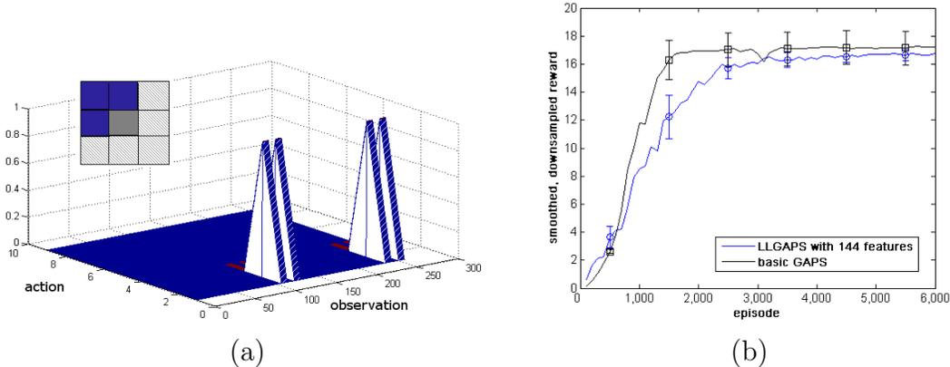
Figure 3-5: 6 modules learning with LLGAPS and 144 features. (a) One of the features used for function approximation in the LLGAPS experiments: this feature function returns 1 if there are neighbors in all three cells of the upper left corner and  $a_t = 2(\text{NE})$ . (b) Smoothed (100-point moving window), downsampled average rewards over 10 runs, with standard error: comparison between original GAPS and LLGAPS.
