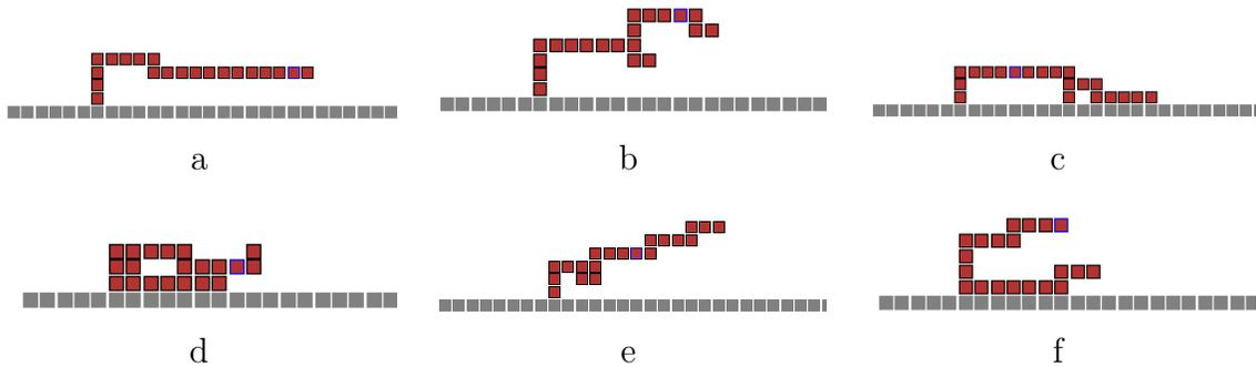
Figure 3-12: Some locally optimal policies result in robot configurations that are not locomotion gaits.
