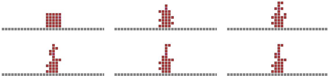
Figure 6-2: A sequence of 25 modules, initially in a square configuration, executing a learned policy that builds a tall tower (frames taken every 5 steps).
