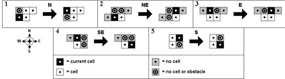
Figure 1-2: A hand-designed rule-based controller for locomotion by self-reconfiguration on a square lattice. Reprinted with permission from Butler et al. (2004).
