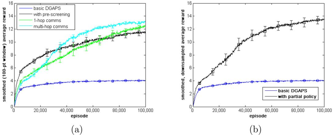
Figure 4-10: Smoothed, downsampled average rewards over 10 trials with 15 modules learning to locomote using only their own experience, with standard error: (a) basic distributed GAPS vs. GAPS with pre-screening for legal motions vs. GAPS with pre-screening and 1-hop (green) or multi-hop (cyan) communications with neighbors below, and (b) basic distributed GAPS vs. GAPS with all actions and a partially specified policy as starting point.
