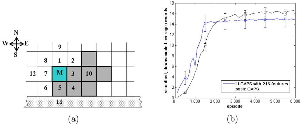
Figure 3-7: (a) During experiments with an extended observation, modules had access to 12 bits of observation as shown here. (b) Smoothed (100 point moving window), downsampled average rewards obtained by 6 modules over 10 trials, with standard error: comparison between basic GAPS and LLGAPS.
