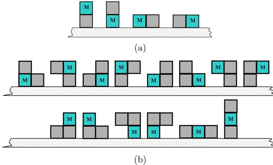
Figure 3-15: All possible local observations for (a) two modules, and (b) three modules, other than those in (a).
