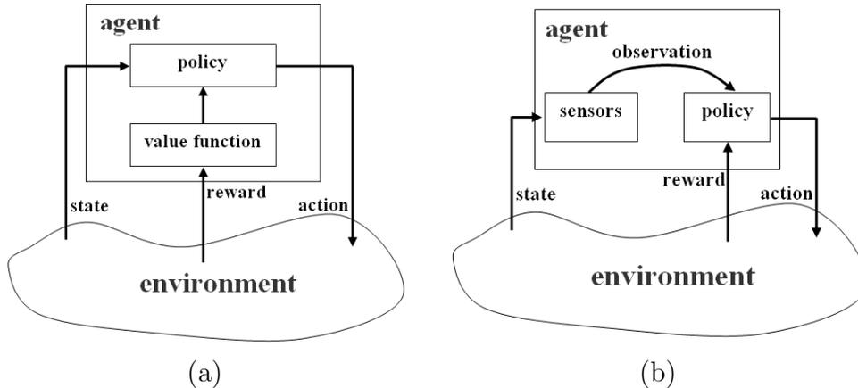
Figure 1-3: The reinforcement learning framework. (a) In a fully observable world, the agent can estimate a value function for each state and use it to select its actions. (b) In a partially observable world, the agent does not know which state it is in due to sensor limitations; instead of a value function, the agent updates its policy parameters directly.
