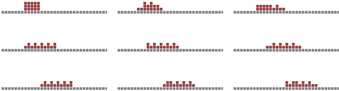
Figure 3-9: Screenshot sequence of 15 modules executing the best policy found by GAPS for eastward locomotion.
