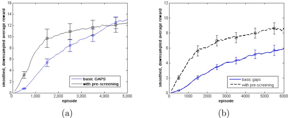
Figure 4-2: Smoothed (100-point moving window), downsampled average rewards comparing the basic GAPS algorithm versus GAPS with pre-screening for actions resulting in legal moves, with standard error: (a) 15 modules (50 trials in basic condition, 30 trials with pre-screening), (b) 20 modules (20 trials in each condition).
