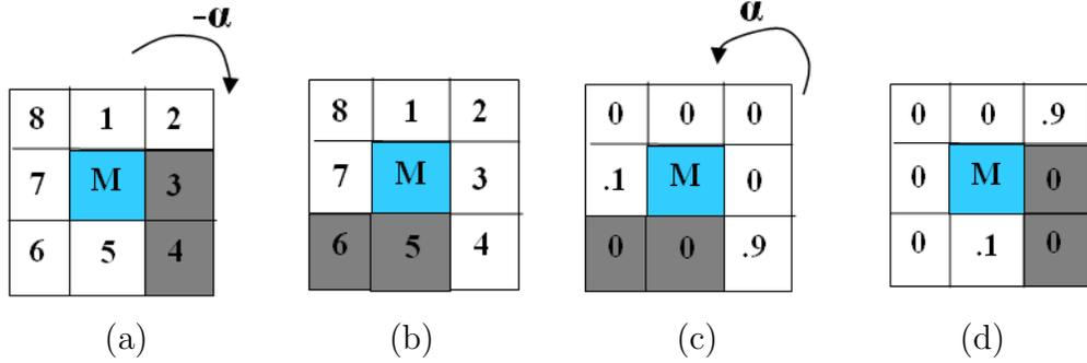
Figure 6-8: Policy transformation with standard GAPS representation when the reward direction is rotated by  $\pi/2$  from the horizontal (i.e., the modules now need to go North, but they only know how to go East): (a) find local neighborhood and rotate it by  $-\pi/2$  (b)-(c) the resulting observation generates a policy (d) rotate policy back by  $\pi/2$  to get equivalent policy for moving North.
