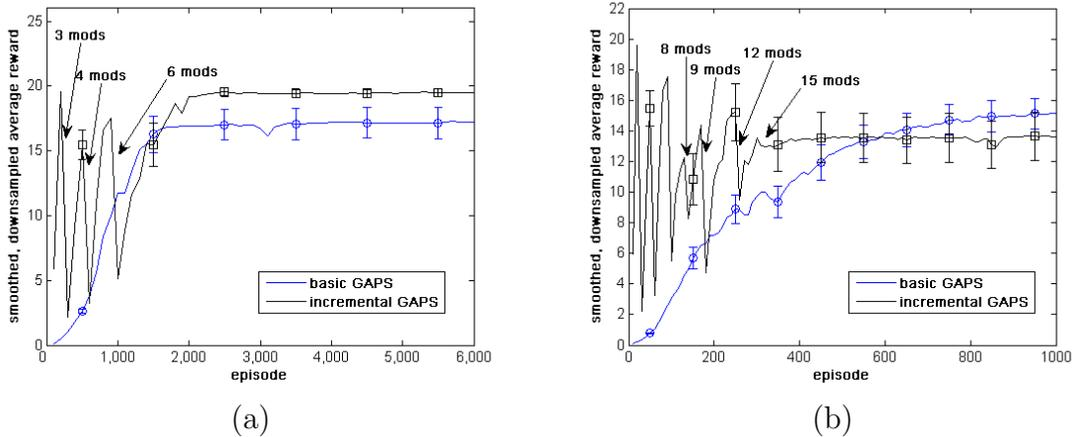
Figure 4-6: Smoothed, downsampled average rewards, with standard error, over 10 trials: comparison between basic GAPS and the incremental extension (a) for 6 modules and (b) for 15 modules.
