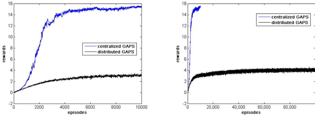
Figure 3-8: Comparison of learning performance between the centralized, factored GAPS and the distributed GAPS (DGAPS) implementations: smoothed (10-point window) average rewards obtained during 10 learning trials with 15 modules. (a) first 10,000 episodes, and (b) to 100,000 episodes of learning.
