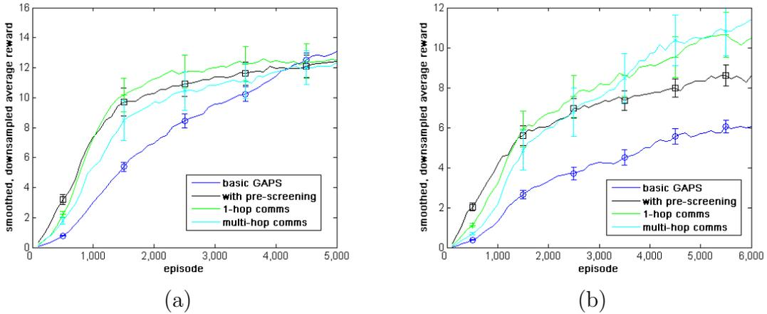
Figure 4-4: Smoothed (100-point window), downsampled average rewards comparing the basic GAPS algorithm to GAPS with pre-screening for legal actions and an extra bit of communicated observation through a 1-hop or a multi-hop protocol, with standard error: (a) for 15 modules (50 basic GAPS trials, 30 GAPS with pre-screening trials, 20 trials each communications), (b) for 20 modules (20 trials each basic GAPS and pre-screening, 10 trials each communications).
