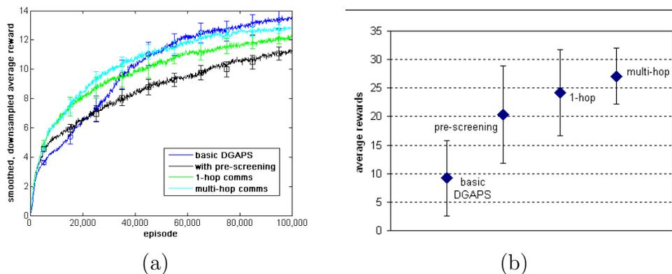
Figure 4-11: (a) Smoothed, downsampled averaged reward over 10 trials of 15 modules running algorithms seeded with a partial policy, with and without pre-screening for legal actions and extra communicated observations, with standard error, (b) Average rewards obtained by 15 modules with episodes of length  $T = 150$  after 100,000 episodes of distributed GAPS learning seeded with partially known policy, with various degrees of constraints and information, with standard deviation.
