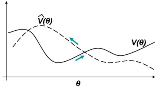
Figure 5-1: Stochastic gradient ascent updates are not necessarily in the direction of the true gradient.
