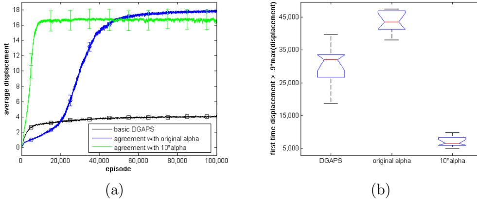
Figure 5-5: Smoothed (100-point window), downsampled average center of mass displacement, with standard error, over 10 runs with 15 modules learning to locomote eastward, as compared to the baseline distributed GAPS. (a) The modules run the agreement algorithm on rewards and experience counters at the end of episodes with original vs. scaled learning rates. (b) Distribution of first occurrences of center of mass displacement greater than 90% of maximal displacement for each group.
