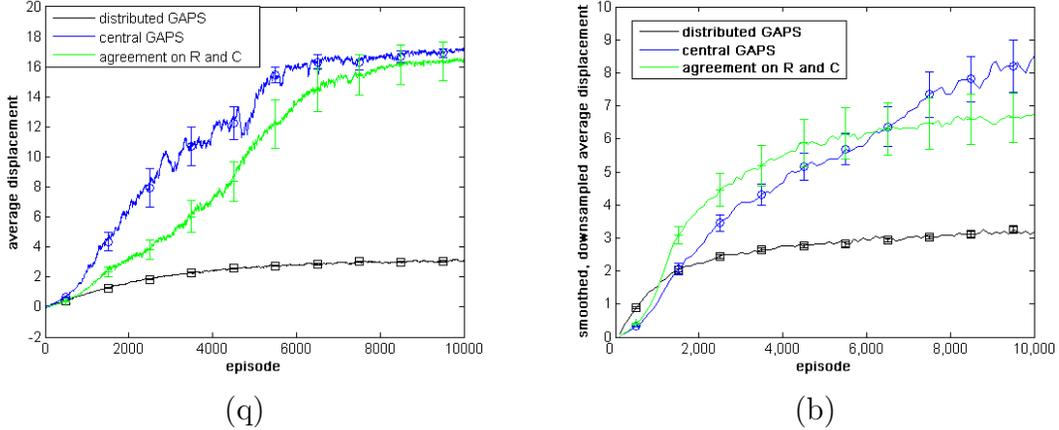
Figure 5-6: Comparison between centralized GAPS, distributed GAPS and distributed GAPS with agreement on experience: (a) smoothed (100-point window) average center of mass displacement over 10 trials with 15 modules learning to locomote eastward ( $T=50$ ), (b) same for 20 modules with episode length  $T=100$ : learning was done starting with  $\alpha = 0.2$  and decreasing it uniformly over the first 1,500 episodes to 0.02.
