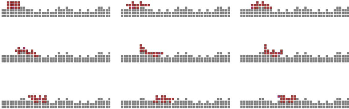
Figure 6-3: First 80 time-steps of executing a policy for locomotion over obstacles, captured in frames every 10 steps (15 modules). The policy was learned with standard-representation GAPS seeded with a partial policy.
