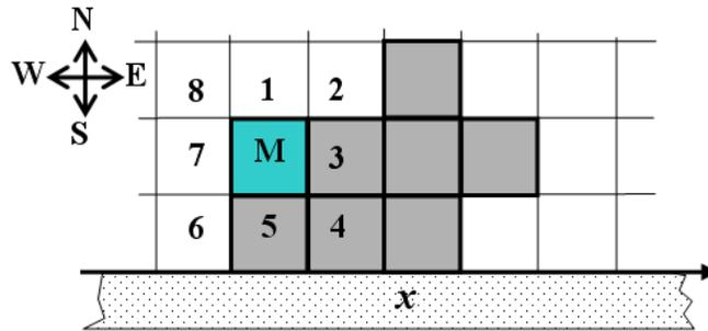
Figure 1-5: The setup for locomotion by self-reconfiguration on a lattice in 2D.
