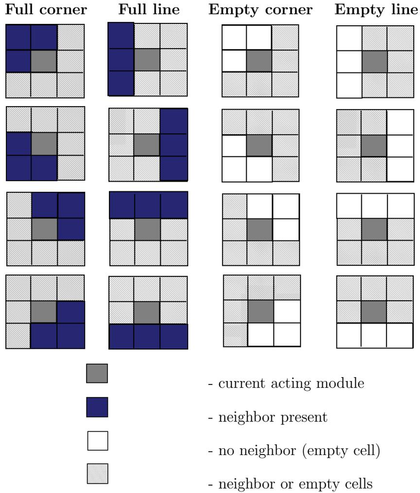
Figure 3-6: All 16 observation masks for feature generation: each mask, combined with one of 9 possible actions, generates one of 144 features describing the space of policies.
