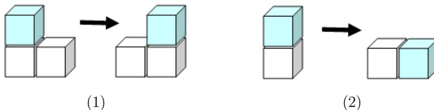
Figure 1-4: The sliding-cube kinematic model for lattice-based modular robots: (1) a sliding transition, and (2) a convex transition.
