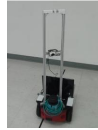
Fig. 8. The experiment setting the monocular camera is mounted on the P3DX platform. The sick laser collects data for laser SLAM as ground truth.
