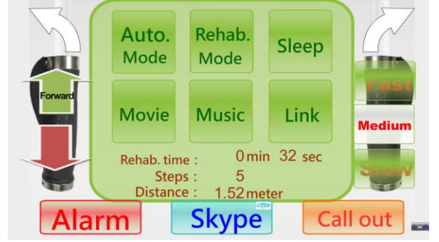
Fig. 5. Touch user interface in rehabilitation mode. On the right, user can set the walking speed to fast, medium or slow. On the left, user can choose either to walk forward or backward. On the bottom, buttons from left to right allow user to sound the alarm, make a skype call and call the care center. In the middle, the three captions from top to down show the elapsed time, total steps and the total distance. The buttons and captions are large enough for elders to choose.
