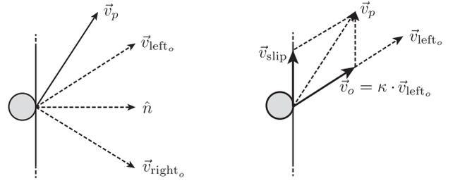
Fig. 6. (left) Probe pushing an object with a velocity  $\vec{v}_p$  outside the motion cone (spanned by  $\vec{v}_{\text{left}_o}$  and  $\vec{v}_{\text{right}_o}$ ). (right) The push results into a motion to the object  $\vec{v}_o$  along the left bound of the motion cone, and sliding of the pusher along the boundary of the object  $\vec{v}_{\text{slip}}$ .
