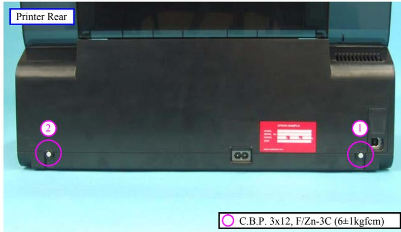
Figure 4-6. Removing Upper Housing (1)
