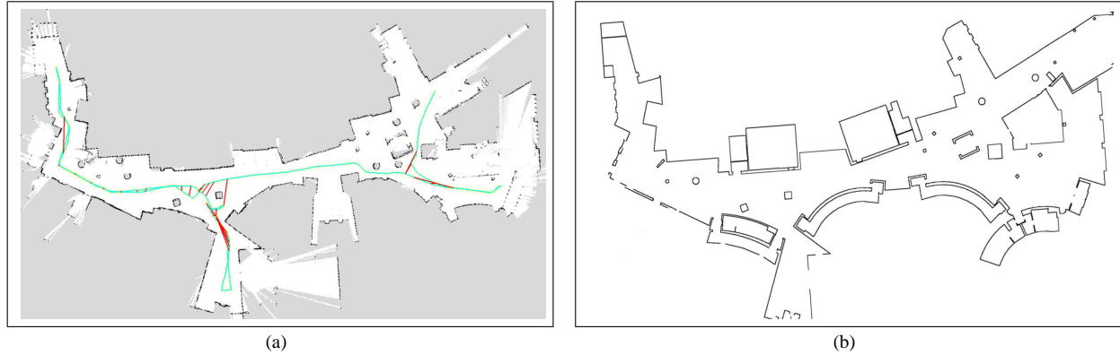
Figure 8: (a) The occupancy map of the first floor of MIT’s Stata center constructed by the vehicle during autonomous flight. The trajectory of the vehicle is shown in cyan, and detected loop closures are drawn in red. (b) The architectural floor plan of the building for comparison purposes.
