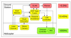
Figure 2. Schematic of our hierarchical sensing, control and planning system. At the base level, the onboard IMU and controller (green) creates a tight feedback loop to stabilize the helicopter's pitch and roll. The yellow modules make up the real-time sensing and control loop that stabilizes the helicopter's pose at the local level and avoids obstacles. Finally, the red modules provide the high-level mapping and planning functionalities.
