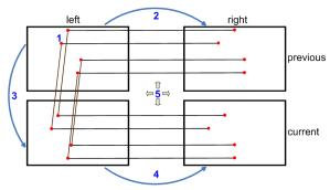
Figure 3. Basic scheme of the stereo visual odometry algorithm: 1. Feature detection; 2. Tracking from *left* to *right* frame and depth reconstruction; 3. Tracking from previous to current frame; 4. Similar to 2.; 5. Frame to frame motion estimation.
