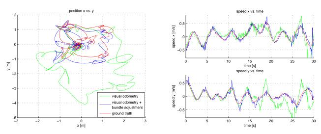
Figure 6. Position and speed over 1200 frames estimated by simple visual odometry from frame to frame (green) and by optimization with bundle adjustment (blue) compared to ground truth (red) obtained by a VICON system. The vehicle was flying with position control based on the estimates from bundle adjustment
