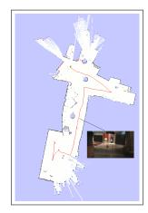
Figure 7. Map of the first floor of MIT's Stata Center constructed by the vehicle during autonomous flight.
