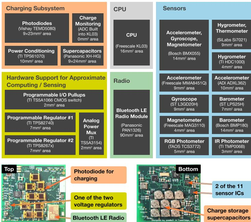
**Figure 1.** Warp hardware platform contains ICs that together provide 21 sensors across eight sensing modalities. Table 1 details the sensors further. Because some sensors have multiple subdimensions (e.g., three-axis accelerometers), Warp provides a total of 35 different sensor signal channels. Warp combines this diversity with circuit support to enable approximate computing tradeoffs between precision, accuracy, performance, and energy-efficiency.
