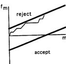
The sequential ratio test defines two lines with different intercepts and the same slope. Above the upper line is a reject region. Below the lower line is the accept region. The test generates a random walk starting at the origin which terminates when it reaches one of the two lines.
