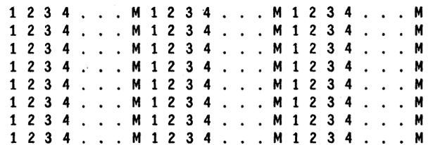
Figure 1. A common organization for raster-graphics memory which is efficient for raster scan operations, but poor for vertical updates.
